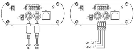
**Note:** Always connect stereo sources to both CH1(L) and CH2(R) inputs to retain full music content. If only one source channel is available, use an RCA y-adapter or jumper wires to connect it to both CH1 and CH2 inputs, otherwise signal level will be reduced by half and require increasing the gain to achieve full power output.
