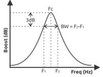
adjustment is 1.5 (wide) to 5 (narrow). To calculate the bandwidth between the -3dB points that are boosted by the EQ band, use the formula BW = Fc/Q.
