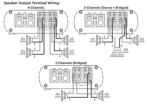
**Note:** After checking all wiring and connections, make all initial settings and adjustments before turning on the amplifier to avoid damaging the connected speakers. Gains should always start at minimum with the appropriate input range selected for your aftermarket or OEM source's maximum output voltage. For smaller speakers, always activate the HP filter and set the cut-off frequency to protect them from being over-driven.
