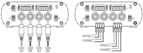
**Note:** For a 2-channel source, connect to CH1/2 inputs and select copy (1/2) with CH3/4's INPUT CH switch. If separate gain control is desired for CH3/4, use RCA y-adapters or jumper wires to connect CH1/2 to CH3/4's inputs externally and select direct (3/4) with CH3/4's INPUT CH switch.
