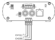
**Note:** Always connect stereo sources to both CH1(L) and CH2(R) inputs to retain full music content. If only one source channel is available, use an RCA y-adapter or jumper wires to connect it to both CH1 and CH2 inputs, otherwise signal level will be reduced by half and require increasing the gain to achieve full power output.
