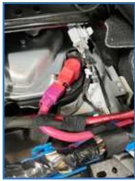
DC-DC "penthouse" lug under rear seat (~15-15.5VDC)
